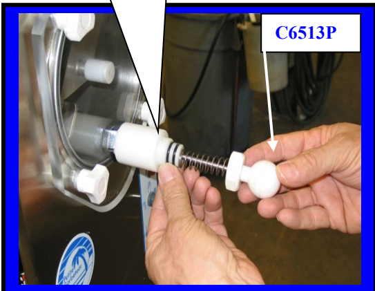
Installing Plunger Assembly into Faucet body
