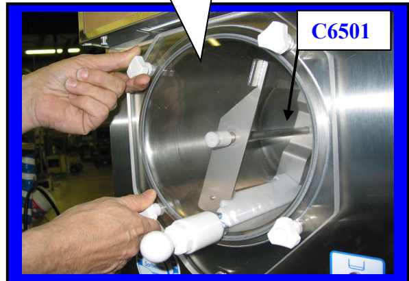
Installing Faceplate onto front of Machine.
