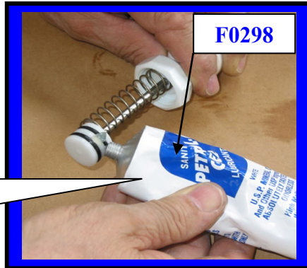
Install O-rings onto plunger
