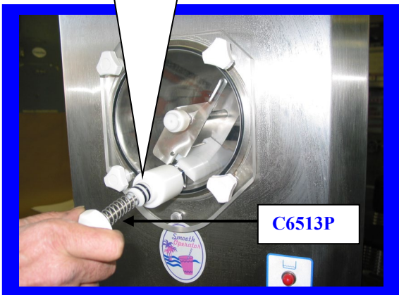
Installing Plunger Assembly into Faucet body
