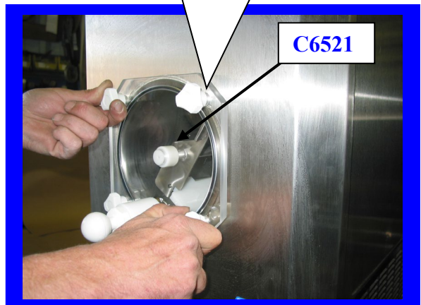
Installing small Faceplate onto front of Machine.
