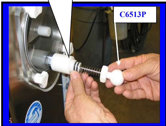
Installing Plunger Assembly into Faucet body
