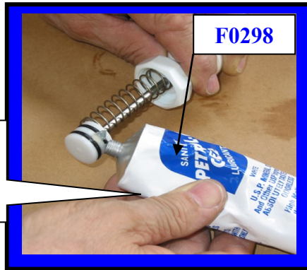
Lubricating O-rings with Petro-Gel
