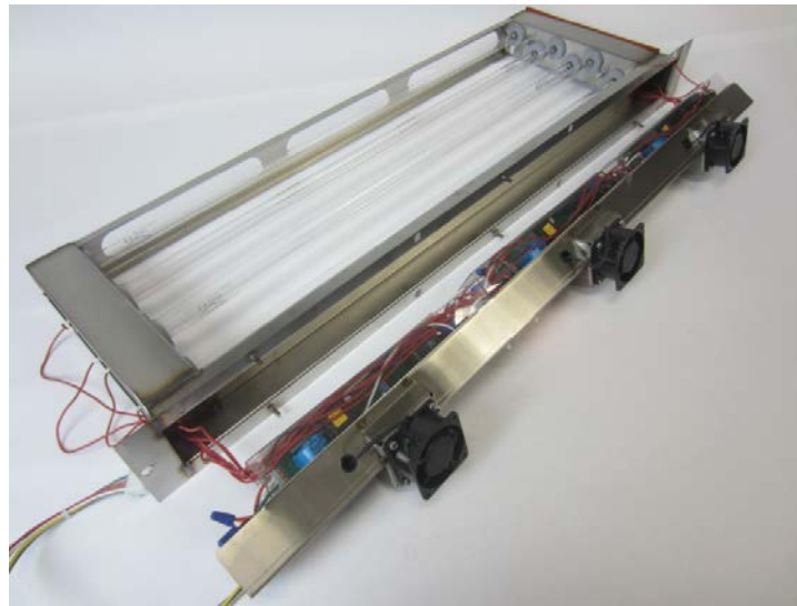
Figure 6-34-2 Ballast Raceway Removed from Module
