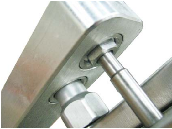
Figure # 5 - No more than two (2) threads female, as per diagram showing above
