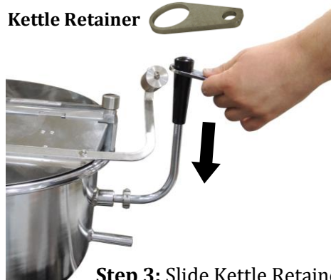
Step 3: Slide Kettle Retainer onto the kettle arm.
