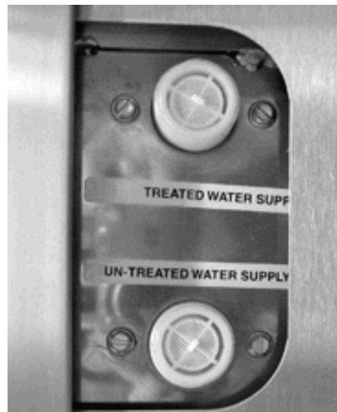
Standard water connections for steam generator and drain spray condenser.
