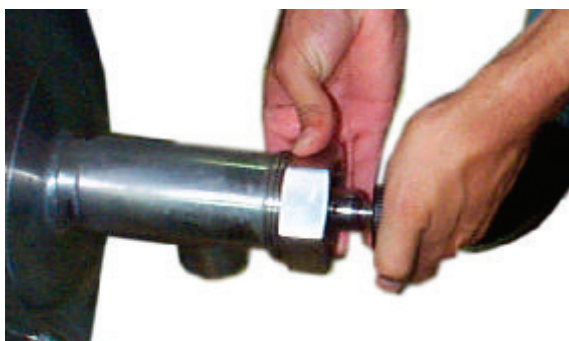
When attaching the draw-off valve hand-tighten the nut.
