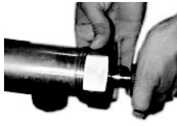
When attaching the draw-off valve, hand-tighten the nut.
