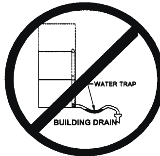
IMPROPER DRAIN LINE CONNECTION
