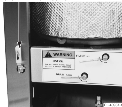
GAS VALVE IN ON POSITION
