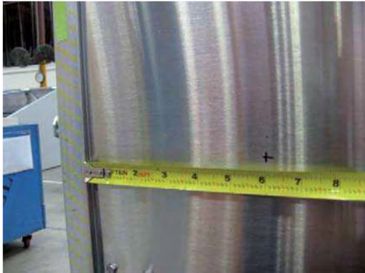
Step 1: Measure 6 inches from wrapping board end.
