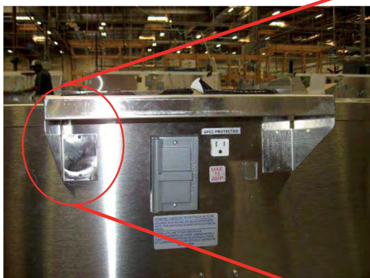
2.- Drill holes and screw in place (with screws provided – Hex Tek S/S 10-16 X 1/2")
