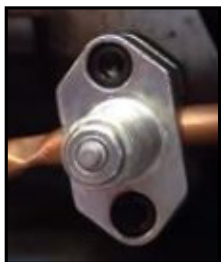
refrigeration line tapping valve
