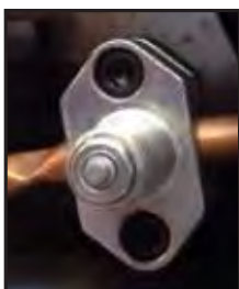
refrigeration line tapping valve
