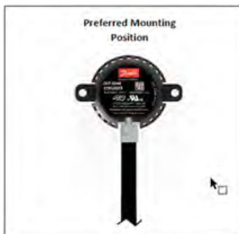
Mount Sensor with cable facing downward if possible. This is to minimize Water ingress from the cable and connector.
