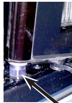
Door must be properly seated inside bottom hinge plate after door tension is applied.
