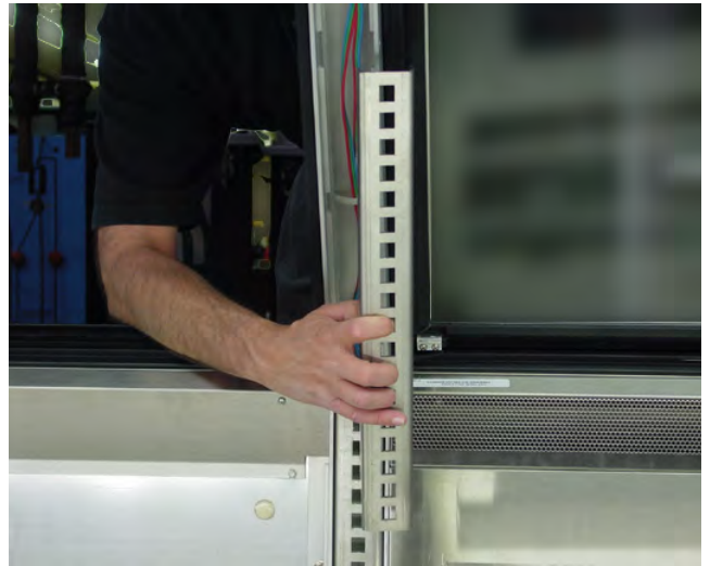
STEP 9 – Lift out upper shelf supports.
