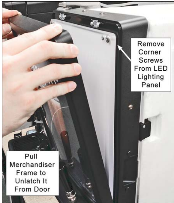
Figure 6-10 - Merchandiser LED Backlight Removal
