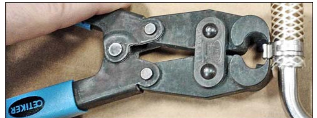
Figure 6-5 - Hose Clamp Removal (Oetiker Tool)
