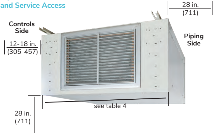
Figure 11. HLY Unit Clearance and Service Access
