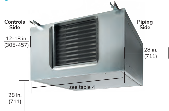
Figure 9. HXY Unit Clearance and Service Access
