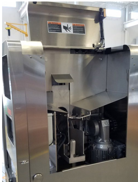
Figure 68. Hopper with Side Access Panel Removed
