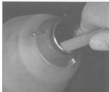
Figure 6a. Sharpening Cutter with Whetstone
