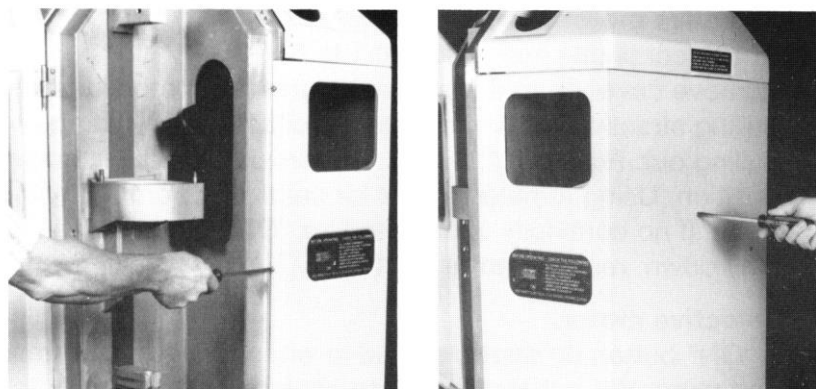
Figure 17. Removal of Switch Cover Panel
