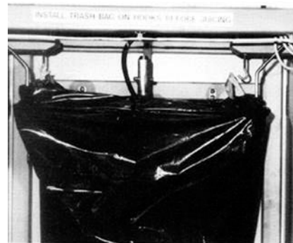
Figure 1f. Trash bag installed
