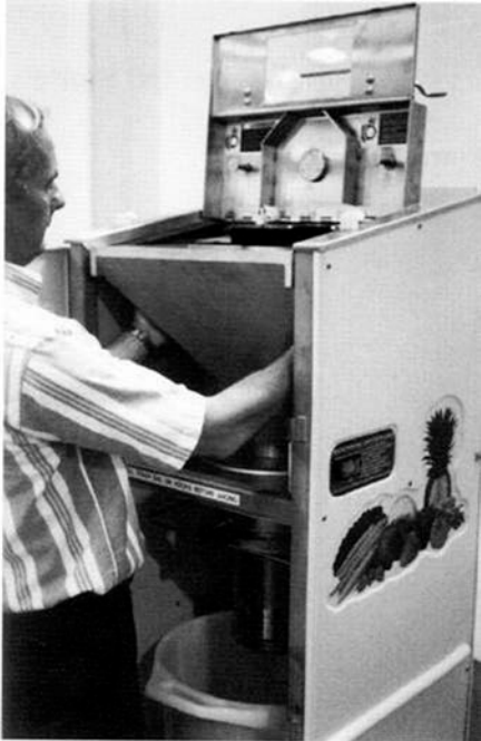
Figure 1c. Lifting out hopper
