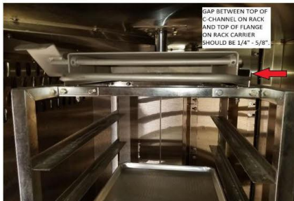
RACK CARRIER HEIGHT AS PROPERLY ADJUSTED
