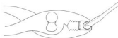
Figure 12 Disconnecting wires at heating elements using pliers to prevent twisting of terminals
