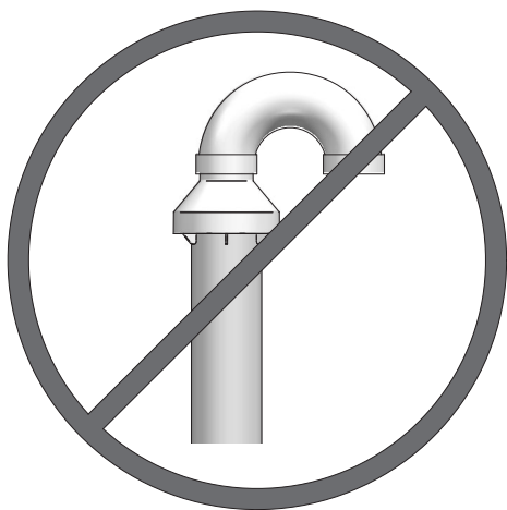
Figure 5-5 Do Not Install U-Bend to Rain Cap
