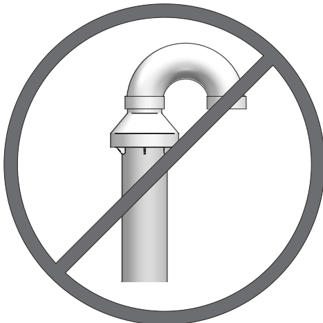
Figure 5-5 Do Not Install U-Bend to Rain Cap
