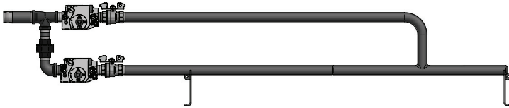
Figure 8-5_Gas Train 500,000 Btu/hr Model
