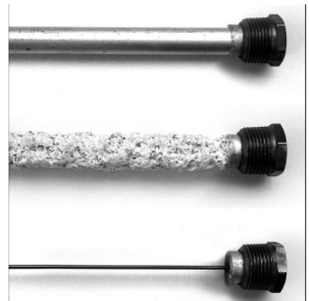
Figure 14 - Anode rods from new to (top) to partially depleted (middle) to fully depleted stages (bottom).
