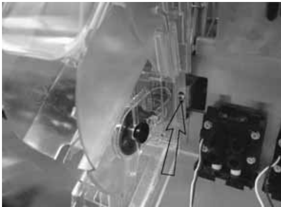
One Adjustment Screw on Each Side of QD Assembly
