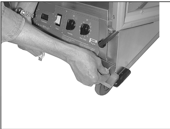
To remove trough: remove thumbscrews; drop trough down and pull forward.
