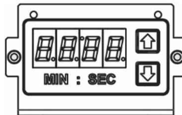
Figure 21. Conveyor Speed Digital Control
