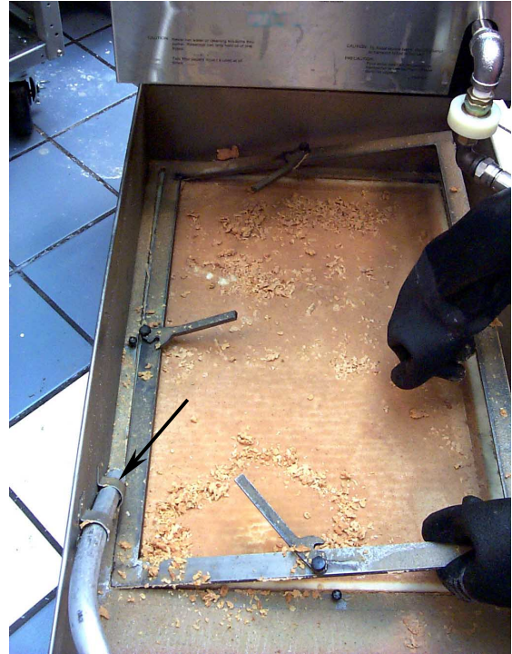
Removing hold-down ring. Note location of wand holster (arrow).
