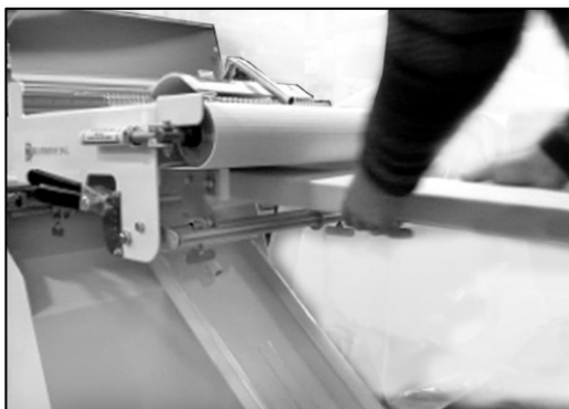
INSTALL PRESSURE PLATE
