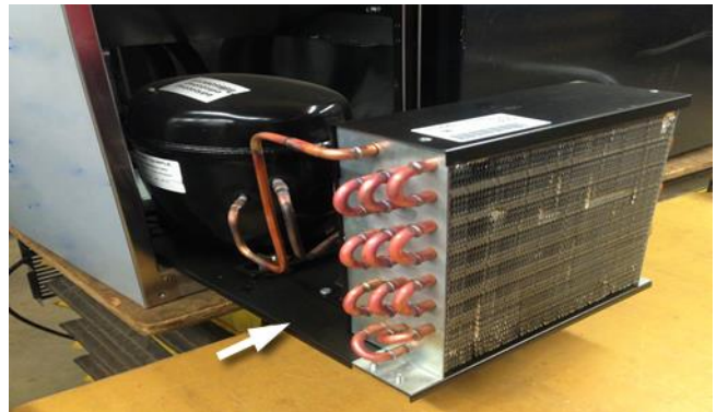
Figure 6-5. Removing Refrigeration Deck
