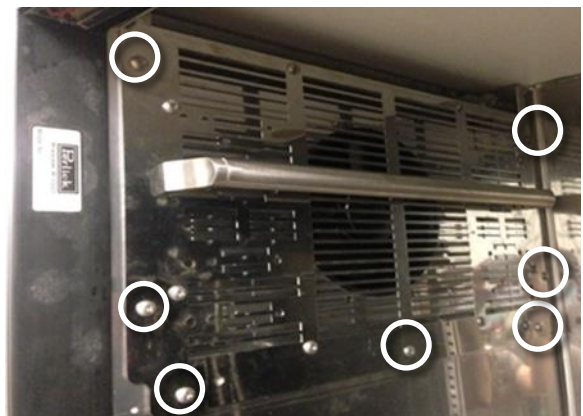
Figure 6-8. Removing Evaporator Fan Panel
