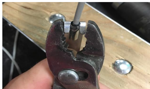
Figure 7-2. Attach Probe to Bracket
