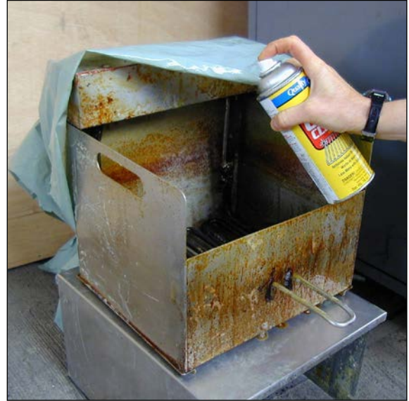
OIL VAT BEING SPRAYED WITH OVEN CLEANER
