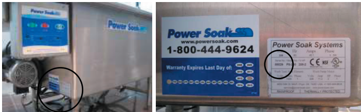
The serial number is 5-6 digits long and located on the lower corner of the wash tank closest to the controller.
