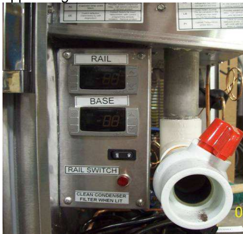
Figure 1 illustrates the outer panel of the mechanical housing. The upper temperature control is for the refrigerated rail and the lower temperature control is for the refrigerated base.
