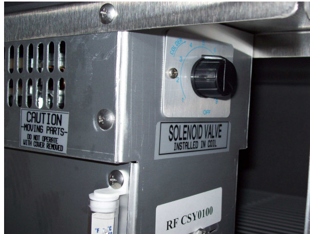
Figure 2 illustrates the evaporator blower coil assembly inside the lower refrigerated base. The thermostat adjustment knob is located at the top, front of the coil assembly.
