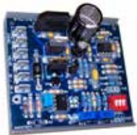
FIGURE 46A - Maxitrol Signal Conditioner, P/N 134170, used in Options AG40, DG2, and DG6
