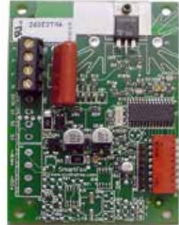
FIGURE 45 - Venter Speed Control Board in Control Options AG8, AG9, AG9H, AG40, AG60, AG61, AG62, DG1, DG2, DG5, DG6, D12B, D12C
