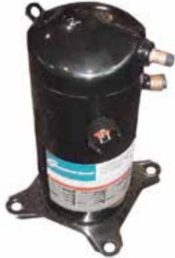
Compressor - Reheat circuit is charged with R410A Refrigerant.
