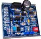
FIGURE 46 - Maxitrol Signal Conditioner, PN 134170 used in Option AG40
