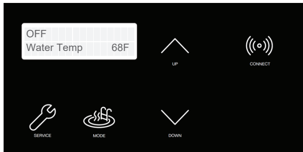
Figure 106. Wi-Fi Reset – Press and Hold CONNECT
