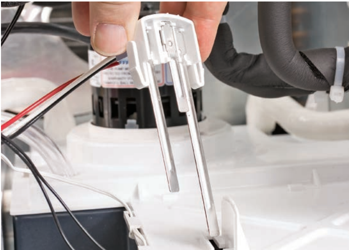
1. Remove Water Level Sensor
