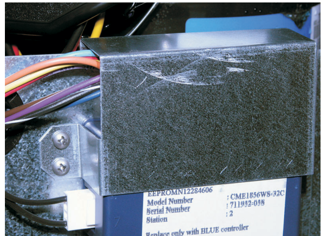
Cover Installed on Unit
