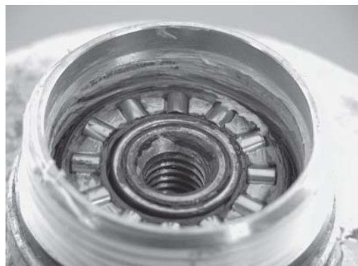
Greased Thrust Half of Bearing
