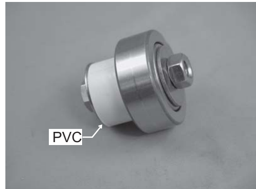
Roller Half of Bearing with insert tool
