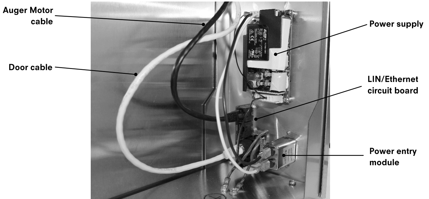
Figure 79: Internal electronics with wiring – multi-row display version
