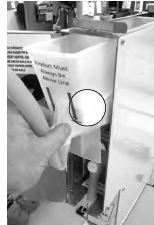
Side of hopper showing locking tab
