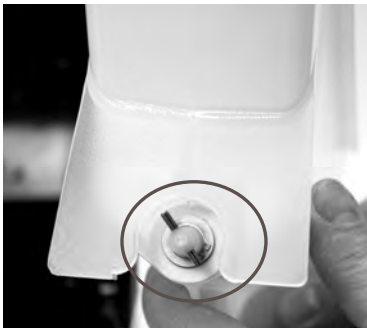
Drive pin on auger at back of hopper
