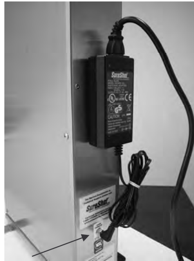
Fasten connector into the receptacle on the back of dispenser
